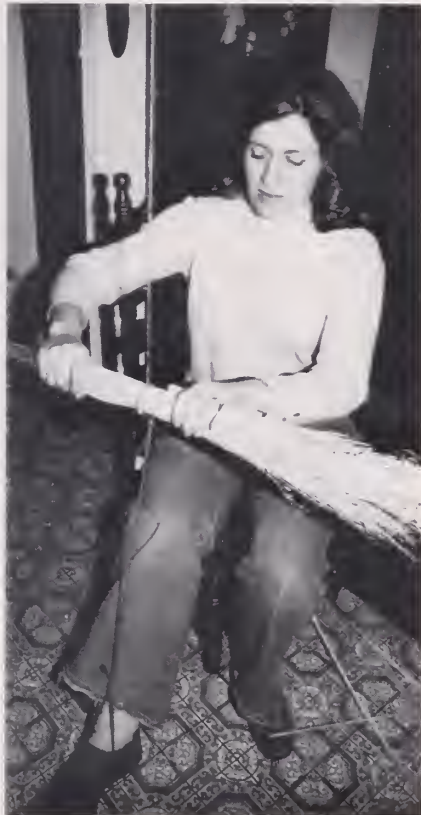
A large nail or hook in the ceiling holds the rope or "third hand" in broom making. Enough slack is needed to wrap this rope around the broom, but then it is kept taut by pressure applied by the foot on the bottom of the rope. Notice the large loop through which the foot is placed.
